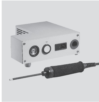
Helium sniffer QUICK-TEST QT 100 with sniffer
